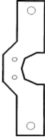
180 Degree Stub Insulator PIN 738-2602 Qty (2) Plastic ID# P2
